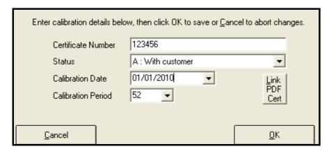
If you have a PDF scanner connected to the computer, ensure the PDF scan is saved to the **C:\ ScanTemp** folder then use the **LINK PDF CERT** button to link the scanned certificate to this job record.
